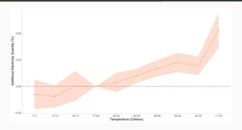
An additional day  $\geq$  35 °C (wrt 17 - 20) increases electricity consumption by 0.53%
